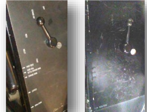
Master Controller Worn vs. New
