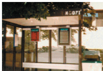
Real time signs mounted inside shelters
