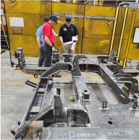
Bogie Frame Inspection
