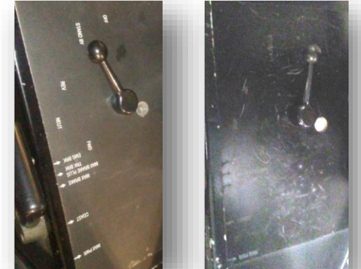
Master Controller Worn vs. New
