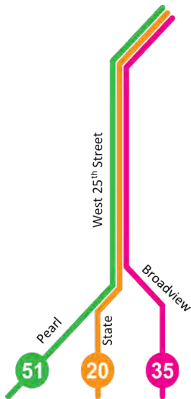
Figure 6: Before 2016, RTA routes 20 (State Road) 35 (Broadview Road) and 51 (Pearl Road) shared the same alignment along West 25 th Street from Broadview Road north to downtown Cleveland, but operated as three separate bus routes. The schedules on the three routes were not coordinated, resulting in highly variable intervals between buses on West 25 th Street.
